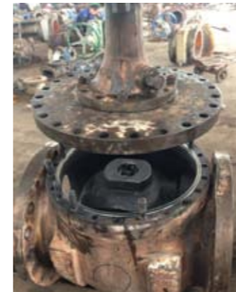
顶装式球阀维修前 Top Entry Ball Valve Before Repair
