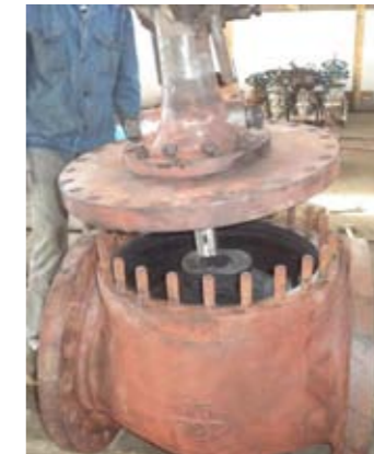
顶装式球阀维修中 Top Entry Ball Valve During Repair
